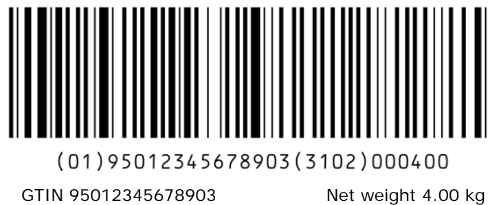
Figure 7.8.5.1-2. Data encoded in one concatenated GS1-128 symbol
