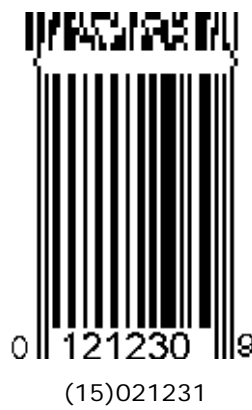
Figure 5.8.8-4. UPC-E symbol with a two-column CC-A
