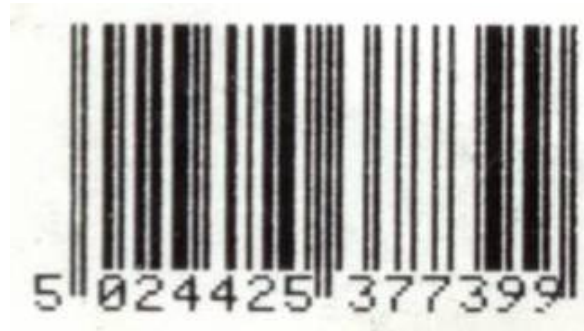
Figure 5.9.5.12-1. Symbol with edge determination problem
