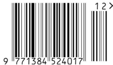
Figure 5.2.2.5.1-2. EAN-13 barcode with two-digit add-on symbol
