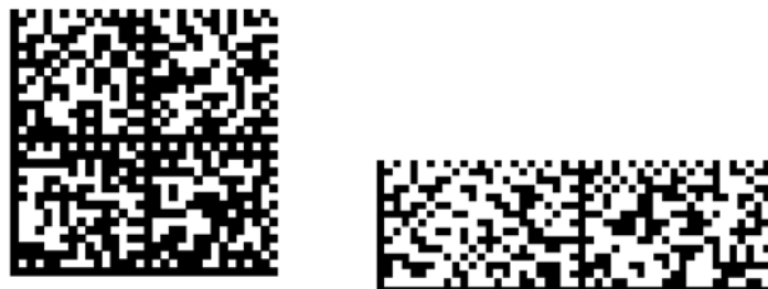
Figure 5.6.3.2-3. Segmented GS1 DataMatrix symbols: Square and rectangular formats (sizes of these GS1 DataMatrix symbols are larger than what would be used in a typical application so that typical alignment patterns can be easily seen.)
