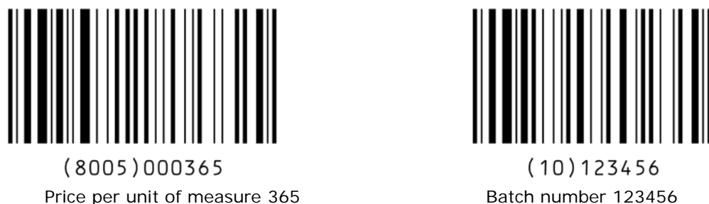
Figure 7.8.5.2-1. Data encoded in two GS1-128 symbols
