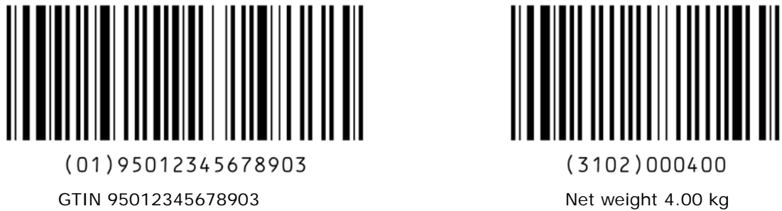
Figure 7.8.5.1-2. Data encoded in one concatenated GS1-128 symbol
