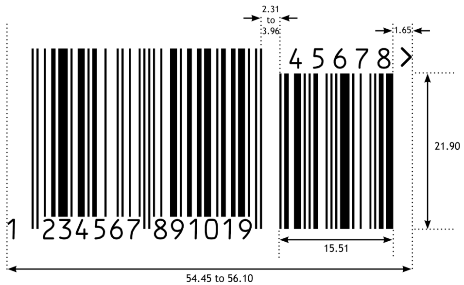
Figure 5.2.6.6-6. EAN-13 barcode with five-digit add-on symbol
