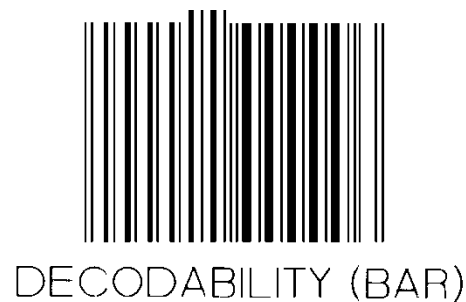
Figure 5.9.5.12-3. Calibration symbol with engineered low decodability grade
