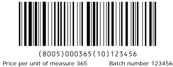
Figure 7.8.5.2-2. Data encoded in one concatenated GS1-128 symbol
