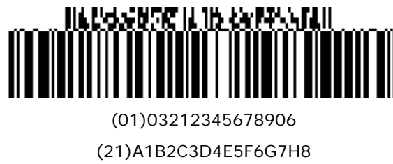
Figure 5.8.8-9. GS1-128 symbol with a four-column CC-A
