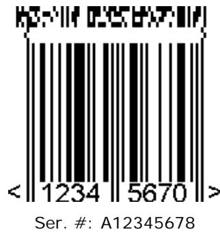
Figure 5.8.8-3. EAN-8 symbol with a three-column CC-A
