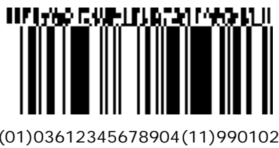
Figure 5.8.8-5. GS1 DataBar Omnidirectional symbol with a four-column CC-A
