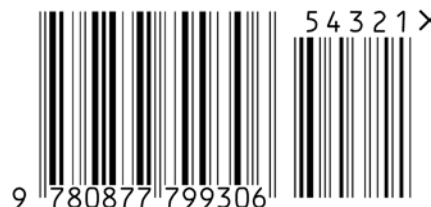
Figure 5.2.2.5.2-2. EAN-13 barcode with five-digit add-on symbol
