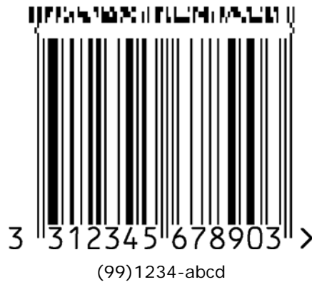
Figure 5.8.8-1. EAN-13 symbol with a four-column CC-A component
